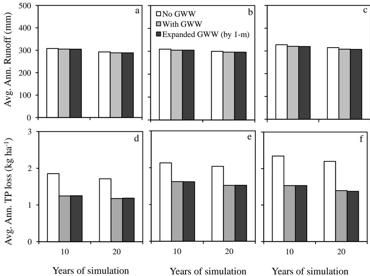
**Figure 3.** APEX model predictions for average annual runoff (a, b, and c) and average annual total phosphorous losses (d, e, and f) for Center, West, and East watersheds, respectively, at the paired watershed study, Greenley Research Center, Missouri, USA, for 10 and 20 years with and without grass waterways and with expanded grass waterway by one meter from all sides.
