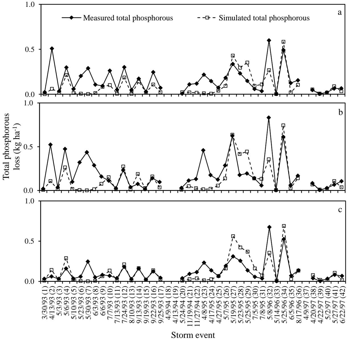
**Figure 2.** Measured and simulated total phosphorous losses for Center (a), West (b), and East (c) watersheds during the study period at the paired watershed study, Greenley Research Center, Missouri, USA. The Center (a) watershed shows the results for calibration while West (b) and East (c) watersheds show the results for validation. Measured total phosphorous for events 18, 19, and 37 were not available.
