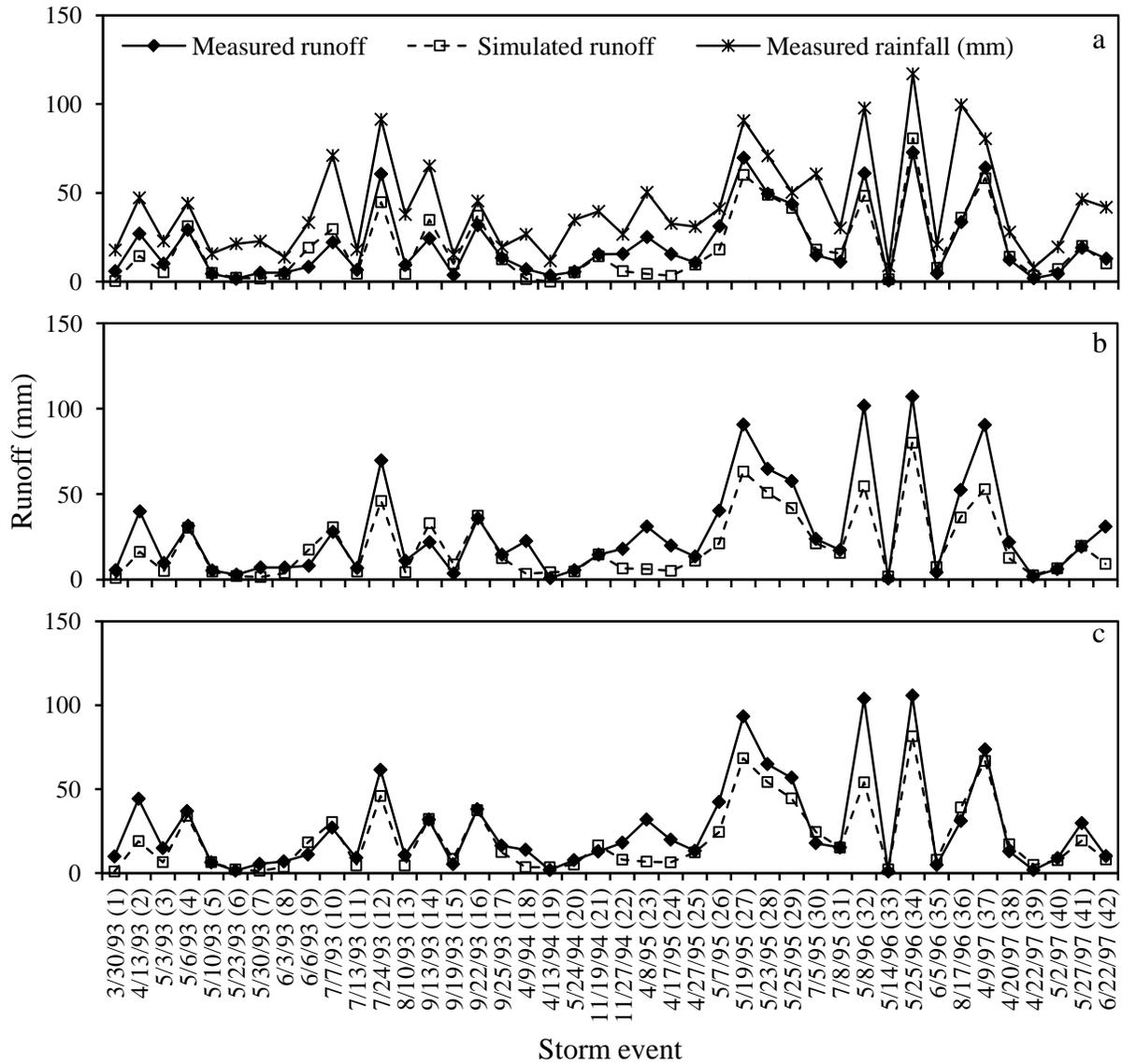
**Figure 1.** Measured and simulated runoff for Center (a), West (b), and East (c) watersheds during the study period at the paired watershed study, Greenley Research Center, Missouri, USA. The Center (a) watershed shows the results for calibration while West (b) and East (c) watersheds show the results for validation.
