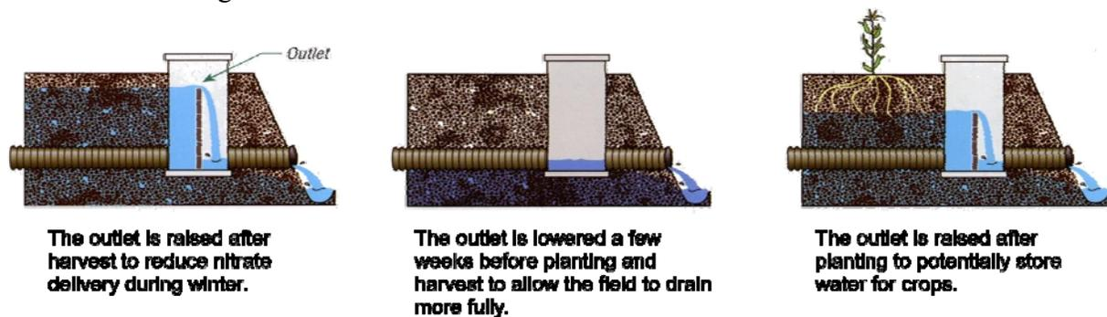
**Figure 1.** An integrated water management system uses controlled drainage to vary the depth of the drainage outlet.
