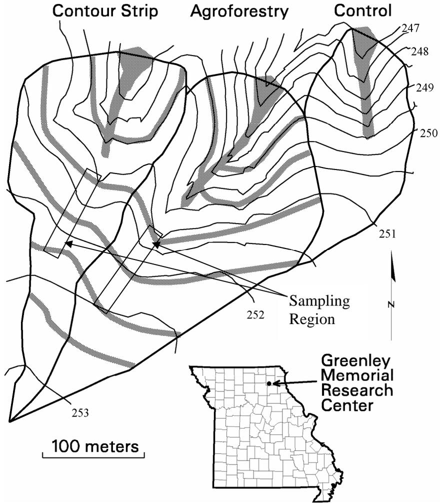
Figure 1. Topographic map of study site with 0.5 m elevation interval contour lines (black), agroforestry buffers (wide gray), grass buffers (wide gray), and sampling region (super imposed box). Grass waterways (wider gray) are located at the outflow end of the three watersheds. Wide gray bands represent tree-grass strips on the agroforestry watershed and grass strips on the contour strip watershed. The inset map shows the location of watershed in Missouri.
